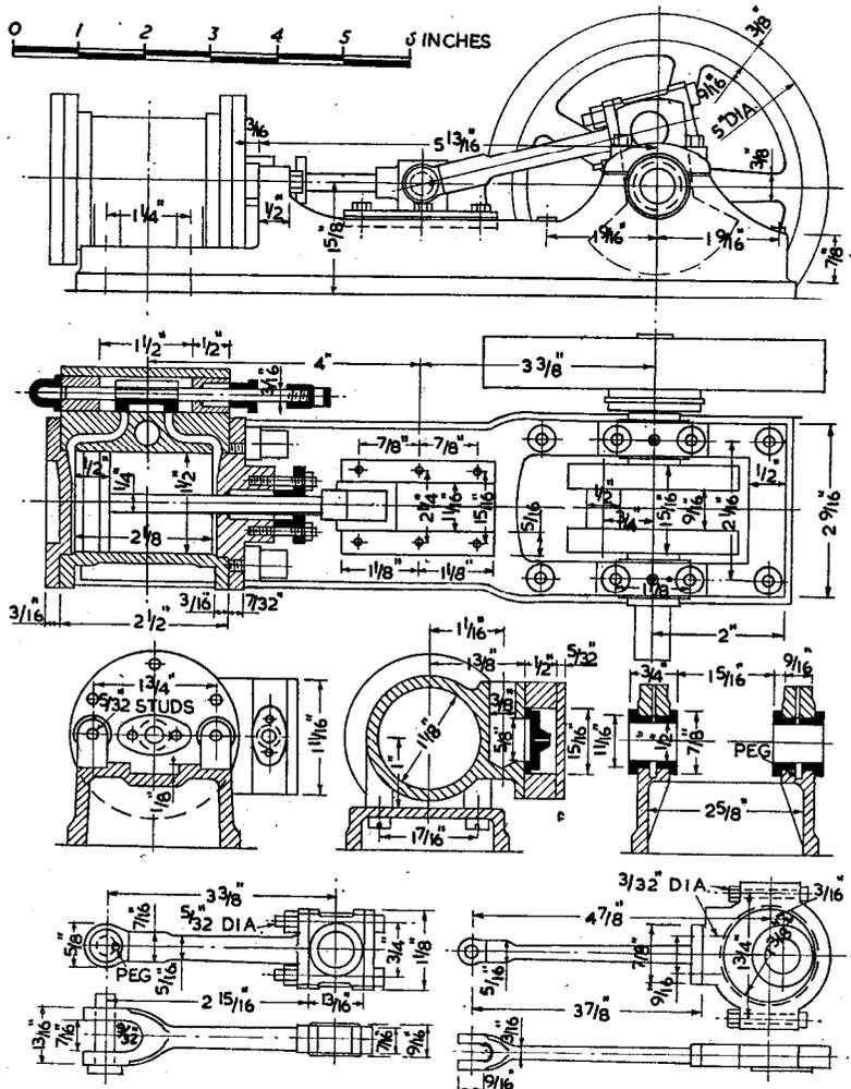
designed by Muncaster, all generally similar in major features but differing in size and certain details. The first, shown in Fig. 18 [March 21], is scaled down from a fairly large engine, 12 in. bore x 18 in. stroke, in the proportion of 1 in. to 1 ft.
