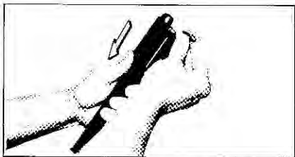
FIG. 1 Pull Down On Loader, Insert Cartridge
