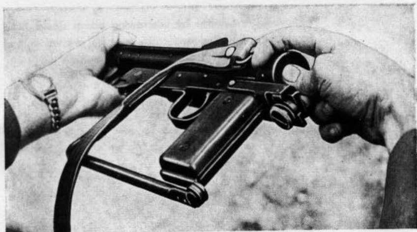
Fig 18. Removing the back piece.
